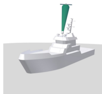
Best location: if possible, place the antenna on top of the boat.
